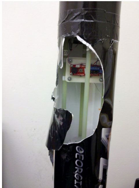
Figure 10: Damage of skin that occurred during landing
