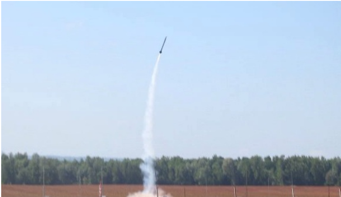
Figure 7: Vehicle weathercocking during launch
