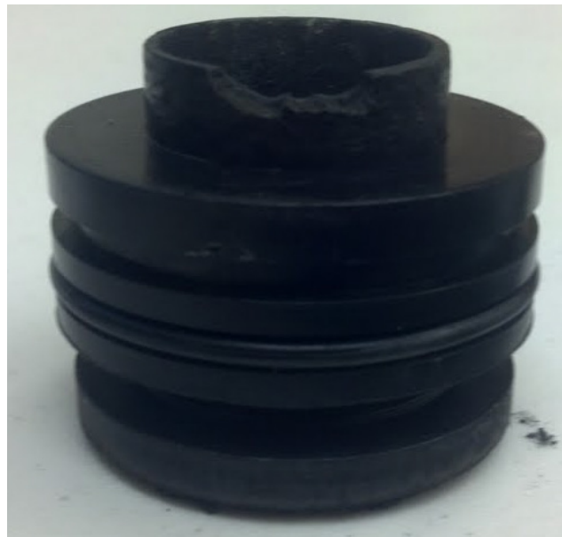
Figure 9: Damage on nozzle
